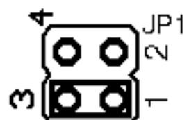
always allows you to take control of any WatchMan and correct any setup errors. The JP1 1-3 jumper also forces the WatchMan into Master Mode Enabled for use on a stand alone bus.
