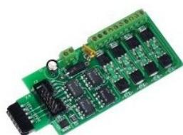
The SCSD-8 Output Module is designed to drive individual solenoid coils or other high voltage high power devices. Normally the input voltage should not exceed 27VDC. The SCSD-8 board is optically isolated from the driving circuitry to protect the Tower LCC+Q or other control device from the high power outputs. When driving single coils or high power loads configure the line as a
