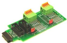
This board is a convenient way to reverse track polarity by using logic in place of Auto Reverse devices. In many cases track polarity may be calculated. In these cases using a DPDT relay is more cost effective and easier on the equipment. Some examples include the tail track of a simple “Y” and the turnout feeding a reverse loop. In both of these cases the required polarity change follows the turnout position.
