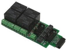
Relay Board - 4 is a Quad 10A SPDT relay board with logic level drivers. It is suitable for use with Tower LCC+Q or other logic level output devices. It requires 12V auxiliary power to drive the relay coils. Auxiliary power is optically isolated from the logic inputs for double isolation. LED indicators for each relay make it easy to monitor activity.
