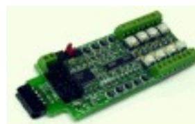
The BOD-8 does not expect you to re-wire your layout to bring track feeders to the detector cards. The small CT (Current Transformer) detection coils are placed directly on the track feeders where they belong. Simple lengths of Cat-5 cable are the usual way to run the signals back to the detector boards. Use of CT coils means that there are no track voltage losses associated with the detectors. Normal detection levels are 1mA. but may be adjusted to higher levels with on board pots.
