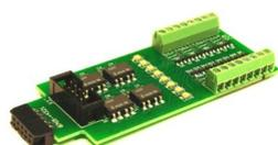
This 8 input board is used when a non-isolated source of voltage needs to be monitored and input to the Tower LCC. One example would be to monitor the DCC voltage on a set of points to determine the position of a turnout without using auxiliary contacts.
