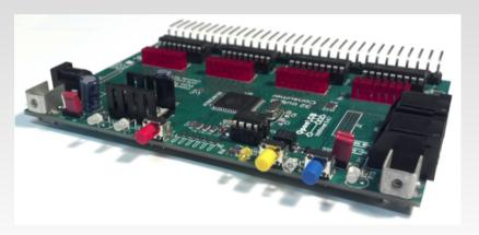
These early boards were essentially OpenLCB replacements for the 32 line Bruce Chubb input and output boards. They were developed as a way for the developers to run real hardware to prove out the specifications. Unfortunately they have the same limitations as their CMRI equivilents in that they are strictly input or output slaves to a computer program. These boards are no longer available nor supported by recent JMRI versions.
